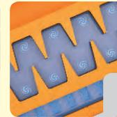
Hydrodynamically designed cascade tooth structure helps to create double flow regime for continuous flushing of dirt.
